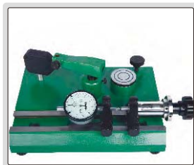
inspect accuracy of dial indicators (range 0-25mm)
